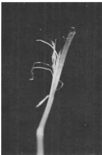
Fig. 8. Fractured end of nucleated, oil-filled dogbone specimen showing fibrillar fracture.
